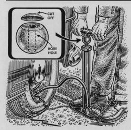
A small rubber ball can be made into a shock absorber for a hand pump. Cut a slice off the ball and drill a hole so that the ball is a snug fit on the pump rod. If the rod bottoms before the ball takes up the shock, shorten the rod slightly.
