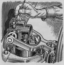
**Clean dirt** from around the filler plug of this type of front shock absorber before attempting to remove the plug. Unless you do, there's a good chance the socket won't go all the way down, you'll round off the plug corners and never get the plug out.
