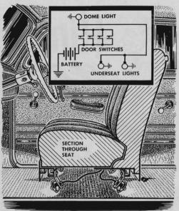
Lights on the floor are a big convenience in a car and easy to install. Get a pair of truck marker lamps, remove the red glass and bolt the lamps under the front seat so one will shine to the front and one to the rear. Wire the lamps as shown so that the door switches will turn them on along with the dome light.
