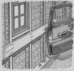
A bumping board placed inside the garrage at the height of the car-door handles will keep the door from being sprung if the car rolls back with the door open. An 8" board placed at handle level will give the driver time for second guesses.
