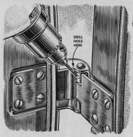
**External hinges** on the doors of old cars often develop a rusty-gate wheeze, and oil squirted on the hinges may do no good. As a remedy, try drilling a small slanting hole near the top of the hinge, going just to the hinge pin. Fill the hole with penetrating oil and let it work down the length of the pin.
