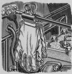
A trucker's gloves will dry as he drives if clipped under the hood like this. A big paper clip astride the radiator support rod is one way to hold them near the hot exhaust manifold. With two pairs along, he can have one pair drving at all times.
