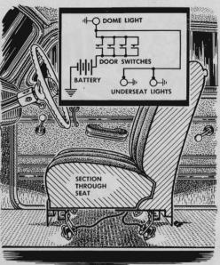
Lights on the floor are a big convenience in a car and easy to install. Get a pair of truck marker lamps, remove the red glass and bolt the lamps under the front seat so one will shine to the front and one to the rear. Wire the lamps as shown so that the door switches will turn them on along with the dome light.
