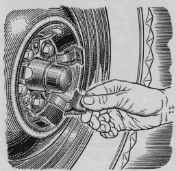
Squeaks may come from the wheels of even a new car. If you have trouble tracking down an elusive running-gear noise, don't neglect the hub caps. In one case, removing the caps and applying a strip of tape on each clip silenced a mysterious chirp.
