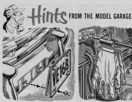
Back up your plates with composition board or exterior-grade plywood to keep the thin metal from becoming banged up in parking scrapes. Run fasteners through plate and board on both edges; use two bottom screws to mount the assembly to the car.
