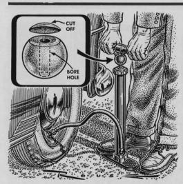
A small rubber ball can be made into a shock absorber for a hand pump. Cut a slice off the ball and drill a hole so that the ball is a snug fit on the pump rod. If the rod bottoms before the ball takes up the slock, shorten the rod slightly.
