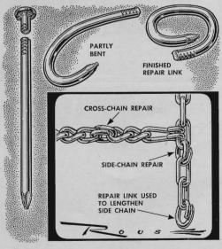
For emergency repair of tire chains, make links from 16-penny nails. Clip off the head and bend the nail as shown, using two pairs of pliers. Leave the opening wide enough so the link can be slipped in place and then bent closed.
