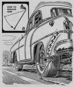
To warn of flat tires, install an extra curb-warning whisker. Bend down the end to ride about halfway between the pavement and the rim of the wheel. Then, the noise as the wire scrapes the ground will let you know the tire has gotten soft.
