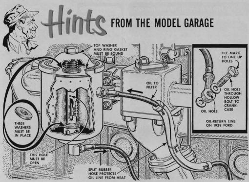
If an oil filter is not working properly you may find the reason or cure here. If the replaceable-cartridge type isn't cleaning the oil, remove the cartridge and make sure the sealing washers, top and bottom, haven't been omitted. Their job is to force oil through the element.
