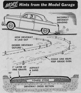
A sharp grade change, perhaps where a driveway joins the street, will cause bumpers and tailpipes to scrape the pavement. So if you are planning a new approach to a garage located above or below street level, lay it out to avoid abrupt grade variations. The sketch shows other helpful points for building a driveway.
