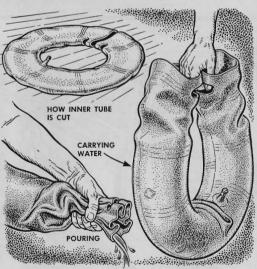
An inner tube cut like this and stowed away in the luggage compartment takes up little space—and will be ready for use if you need a container to carry water.
