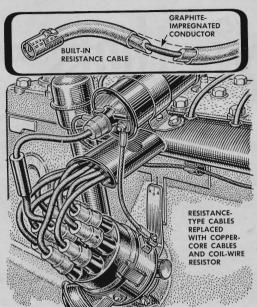
When a tune-up fails to restore an engine's pep, have the ignition cables checked if they are the resistance type. New ones may be needed. Otherwise, you might try the trick of one reader who installed regular stranded cables, put a carbon-type suppressor in the coil wire and found the engine showed marked improvement.
