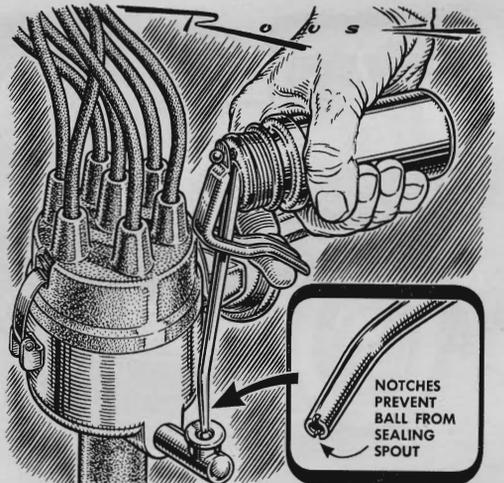
**A notch** filed crosswise in the end of the spout of a pump oiler will help you get oil into ball-check fittings. Otherwise, when the end of the spout is pressed against the ball to depress it, oil may fail to come out—or may squirt to the side.
