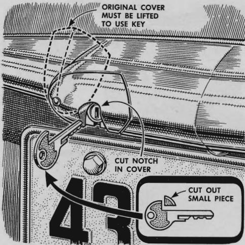
**To open his trunk**, the owner of a late-model Ford reports, it was necessary to hold the lock cover with one hand and turn the key with the other. Modifying the lock cover and key as shown above now permits him to get the lid up with only one hand.
