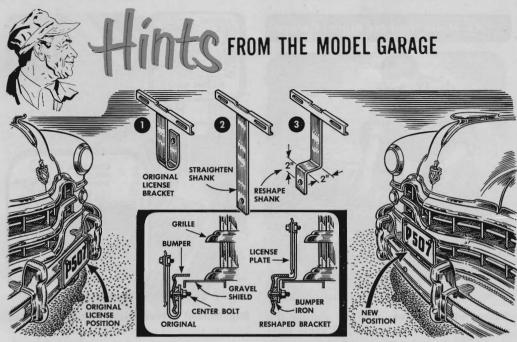
A license plate takes a beating when located ahead of the front bumper. But on some late-model cars that is where the factory bracket forces you to put it.
