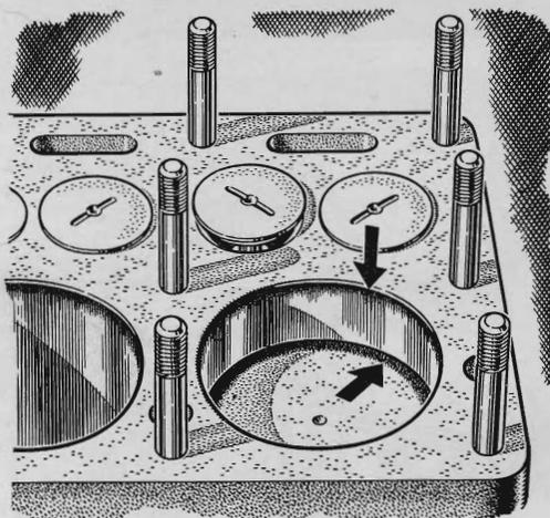
**In scraping carbon** from an engine during a top overhaul, some mechanics contend you can do too good a job. Their practice is to leave a ring about  $\frac{1}{8}$ " wide around the top edge of the piston and another ring around the bore just above piston travel. This, they say, will preserve the oil seal. Removing the carbon may make the car an oil hog.
