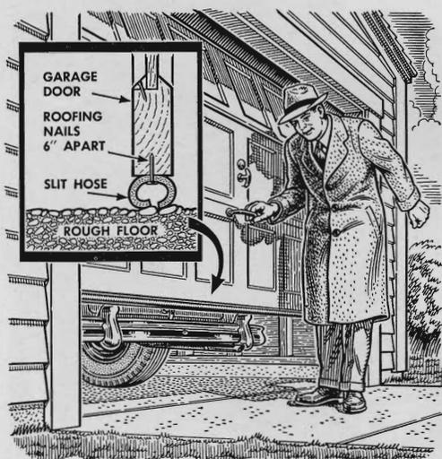
**Cold drafts** can be kept out of a garage fitted with overhead doors by slitting a length of garden hose and nailing it to the bottom edge of the door. This will seal the opening even if the floor of the garage is uneven.
