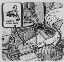
When draining coolant in cold weather, be sure a good stream runs freely from the block or you may have a costly freeze-up. If the water just dribbles out, remove the cock and use the blast from an air hose to loosen the sediment that can block drainage.
