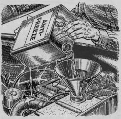
To pour antifreeze into the radiator from a large can, stand at the side of the car with the can extending into the engine compartment so that any dribbles get on the engine and not the body. The fluid won't hunt engine parts, but damages paint.
