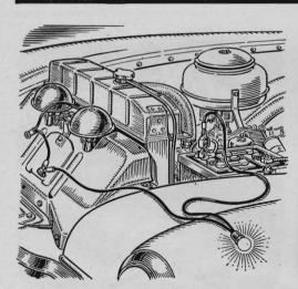
In repairing horn wiring, you can avoid the annoyance of frequent test blasts if you disconnect the wire leading to the horns and connect a test lamp to it and the battery. Use long leads to place the test lamp where it can be seen easily.
