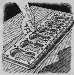
Check a new cylinder-head gasket before installing by matching it with the old one. If they are not identical, a vital water passage might be sealed off with disastrous results. Also, a black area on an old gasket indicates it has not been gastight. So be sure to tighten the head nuts according to specifications.
