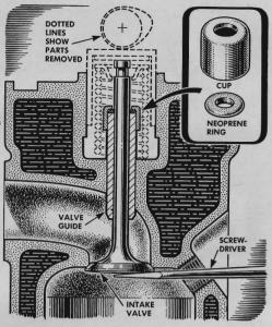
Oil consumption can be cut in a Crosley engine that has a cast-iron cylinder block by installing intake-valve seals just developed by the company. By removing the parts indicated, you can slip the neoprene sealing ring and steel retaining cup down against the guide. A screwdriver through the spark-plug hole will hold the valve up.
