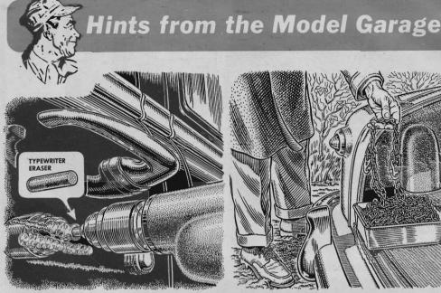
Chucked in an electric drill, the gritty core of a pencil-type typewriter eraser makes it easy to touch up tiny rust spots on a car body without scratching the adjoining paint. The eraser will quickly remove the rust and clean the metal for painting.
