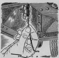
**Drain holes** in the base of a whip antenna sometimes get plugged with dirt, letting water accumulate in the tube. Poking a stiff wire through the holes will release the water and prevent possible interference with the operation of the radio.
