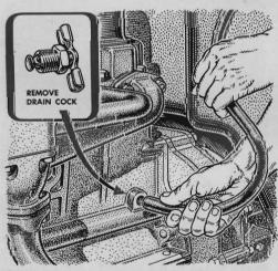
When draining coolant in cold weather, be sure a good stream runs freely from the block or you may have a costly freeze-up. If the water just dribbles out, remove the cock and use the blast from an air hose to loosen the sediment that can block drainage.
