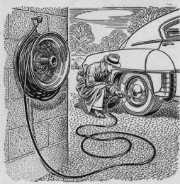
An air-hose hanger for the service station can be quickly made from an old car wheel. Bolt it to the side of the building at waist height. This will keep the hose off the ground and make it easy to unwrap and replace after use.
