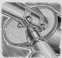
If you can't loosen a bolt holding a muffler or hose clamp and there is no space to use a hacksaw or chisel, try this: Drill a small hole through the side of the bolt and follow it with a bigger drill. Then twist the bolt off.
