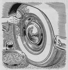
White sidewalls are waxed in the factory to keep the rubber from checking and cracking. Under a hot sun, excess wax may bleed to the surface of a new tire, a condition known as wax bloom. This excess wax should be removed with water, scouring powder and an ordinary scrubbing brush to prevent discoloration of the tire.
