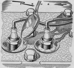
**Compression leaks** around spark plugs can be easily located by sprinkling a liberal amount of talcum powder in the wells and noting any powder disturbance when the engine is started. To eliminate leaks you find, tighten the plugs or replace the gaskets.
