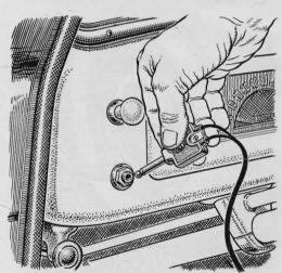
A phone jack of the open-circuit type on the instrument panel makes it easy to connect a home battery charger. Ground one side of the jack and hook the other to the ammeter. Be sure to polarize the charger leads when you connect them to the plug.
