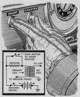
Hot sparks for cold starts can be assured with a setup like this. A Ford coil that uses a resistor in the primary lead is substituted for the regular coil. A normally off pushbutton switch on the dash is depressed at the same time you hit the starter. This bypasses the resistor, giving higher voltage at the coil input.
