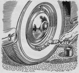
After your wheels are balanced, thev'll look better if you paint the balancing weights the same color as the wheels. A small can of matching touch-up paint will do the job quickly. At the same time, touch up any marks or scratches on the wheels, too.
