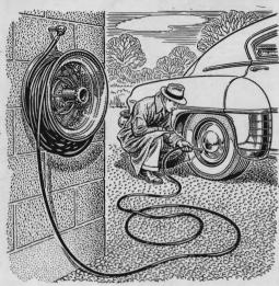
An air-hose hanger for the service station can be quickly made from an old car wheel. Bolt it to the side of the building at waist height. This will keep the hose off the ground and make it easy to unwrap and replace after use.
