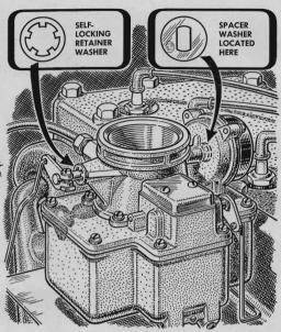
A buzzing carburetor can sometimes be traced to a vibrating choke valve. In the type of carburetor shown (with a spacer washer on the choke shaft), the noise can usually be stopped by seating the retainer washer tight against the air horn, but without causing binding. The lock washer must be placed with its prongs inclined outward.
