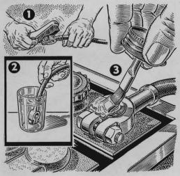
Rubber Cement Saves Battery. Irving J. Covert, Tarpon Springs, Fla., suggests this way to stop corrosion: wire-brush the clamps and terminals, dip them into or wipe on a baking-soda solution, and finally coat the terminal well with rubber cement.
