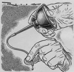
A long flexible extension on the spout of your oilcan will enable you to squirt oil into tight spots where the can itself wouldn't go. A length of model-airplane fuel line (neoprene) is just the right size and the oil won't damage it.
