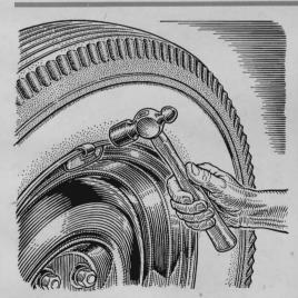
Seat Wheel Weights Carefully. When balancing a wheel, hold the weight in the correct position and give it one or two taps with a light hammer. Hitting too hard may crack the weight or tab. Centrifugal force at high speeds then will loosen it.
