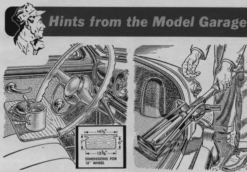
Lunch at the Wheel. For picnicking or eating at a drive-in, a tray like this will often be handy. Gravity and the protruding ears lock it to the wheel. For the other side of the car, the lowered glove-compartment lid makes a useful shelf.
