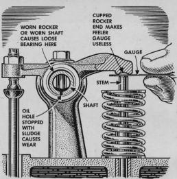
Things to look for in overcoming rough idle, noise or poor performance in an overhead-valve engine are suggested here. An oil-feed line plugged with sludge may cause wear of the rocker-arm bushing and shaft. Severe wear prevents accurate valve timing and proper clearances. The rocker-tip contact surface must be flat.
