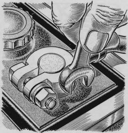
Battery Clamp Easier to Remove. A couple of fiber washers placed between the nut and clamp when you connect a battery cable should make the cable easier to remove later. The washers will help keep corrosion from freezing the nut to the clamp.
