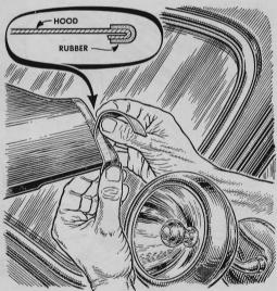
**Hood Pad Protects Spotlight.** If your spotlight swings to a position where the opened hood will strike it, pad the hood edge with a strip of rubber cemented in place. The hood then won't cause any damage if it accidentally hits the spot.
