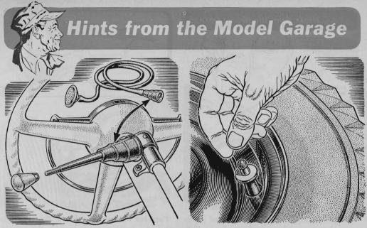
Quieting a Gear Lever. In some older cars, a rattling shift lever on the steering post can be quieted by slipping on one of the rubber hose fittings that come with bathtub sprayers. Force it over the lever and against the steering column.
