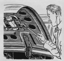
For a neater trunk, stretch a pair of door springs across the inside of the lid, hooking the ends into existing holes. You can then store miscellaneous equipment there-small tools wrapped in cleaning cloths, work gloves and so on. Wire the springs to the lid at intervals to provide compartments for specific items.
