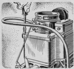
Stalling or rough idling may be caused by air sucked in around the gasket between air-horn assembly and float bowl or carburetor body. Tighten hold-down screws periodically, and also check on the nuts that hold the carburetor to manifold.
