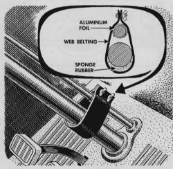
To stop vibration noise in a shift rod paralleling the steering column, try this trick. Belting from surplus army equipment is ideal, for it contains reinforced eyes every few inches. Run small bolts through these. Aluminum foil around the rod acts as a lubricant. The rubber allows a certain amount of give.
