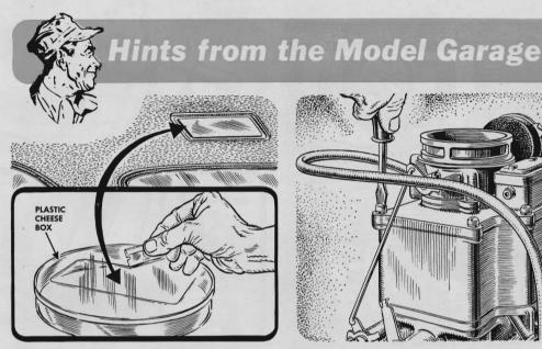
A broken dome-light glass can be replaced easily and inexpensively by cutting the desired size from one of the plastic containers in which cheese and other products are sold. Give the disk a frosted appearance by sanding it lightly.
