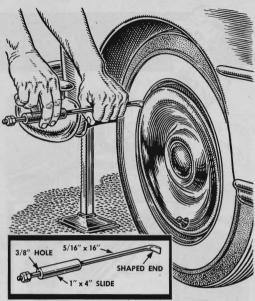
A hub cap will come off easier and there will be less chance of marring the wheel paint if you make a tool like this and add it to your car kit. Ramming the slide against the nut while the hook is under the cap rim does the trick. The tool can also be used to remove front-wheel bearing caps that are pressed in place.
