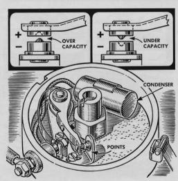
**Pits in distributor points** are a sign that the condenser is of the wrong value. If the positive point pits and the negative one builds up, the condenser is probably over capacity. If it's the other way, the condenser value is too low.
