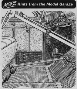
Changing a front tire will be safer and the wheel won't revolve if you first set the brakes with this broomstick arrangement. Cut the stick to the correct length, put a crutch tip on one end and loop cord through a hole in the other. While a front wheel is jacked up you then will have the safety of three locked wheels instead of only two.
