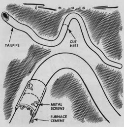
A tailpipe sometimes has so many twists and turns that putting a new one in place becomes a problem. If nothing else works, it may help to saw the pipe in two and later, after the parts are in place, join them with a metal sleeve and furnace cement.
