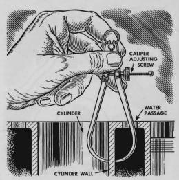
While reboring a cylinder, you can measure the wall with calipers. Put one prong through the water passage and turn up the calipers. Mark the screw setting with a fine pin, take out the calipers, reset the screw and measure between the points.
