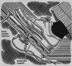
Carpet bunched under the accelerator may make it difficult or impossible to kick down an overdrive transmission from fourth to third to get maximum power. The owner of a car with an automatic transmission may have similar trouble because the pedal is set so low that it bottoms before operating the down-shift switch.
