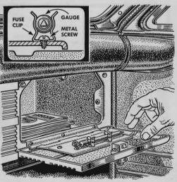
A tire gauge mounted on the inside of the glove-compartment door with a pair of fuse clips will not get lost among the odds and ends in the compartment. Spring clips suitable for the purpose usually cost only a nickel apiece. Fasten with screws.
