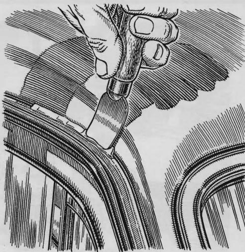
**Calking Protects Eave Trough.** If the original calking falls out of the eave-trough joint on your car, replace it with knife-grade compound and paint the compound a matching color. Water will collect in seams left open, causing rust.
