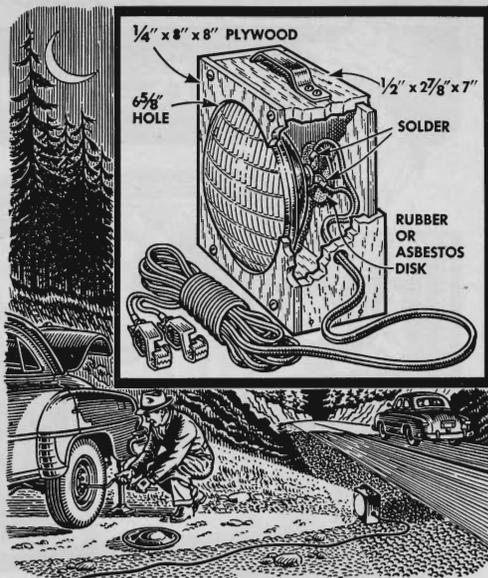
**Lamp for Roadside Emergencies.** When one beam of a sealed-reflector headlamp goes kaput, pack the unit into a box and carry it for night tire-changing and such. Test the three prongs on the back of the lamp to find which two give light. Solder a 15' lead to these. Clamp lamp between box front and the rubber disk.
