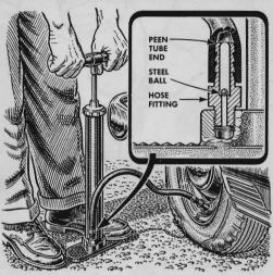
Ball Check Speeds Tire Pumping. An ordinary tire pump may be hard to use if air leaks back from the tire. David R. Fay of Buffalo overcame this by installing a ball check. The ball used was obtained from an old bicycle-wheel bearing.
