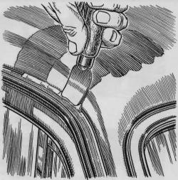
**Calking Protects Eave Trough.** If the original calking falls out of the eave-trough joint on your car, replace it with knifegrade compound and paint the compound a matching color. Water will collect in seams left open, causing rust.
