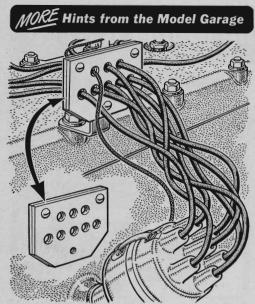
**Tile Prevents Shorts.** An ignition-wire support can be made from two layers of compressed floor tile. Since the tile is an insulator, this is less likely than a metal bracket to cause shorts if insulation wears.
