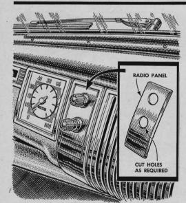
Put Radio Panel to Work. If your car has no radio, you can use the blank panel as a mounting place for accessory switches that you add to the car. Remove the panel and drill or cut out necessary holes. Carefully done, this will look better than switches simply clamped under the dash.
