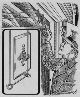
Cords Control Garage Light. In an attached garage that has a light switch only at the house entrance, a cord arranged like this will enable you to turn the light on or off from the garage door.
