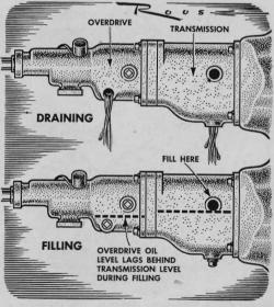
Fill Overdrive Slowly. In some overdrive units, the fill plug is lower than the transmission fill plug. Hence, to get enough lubricant into both units the lubricant should be pumped into the transmission and allowed to flow into the overdrive. Do this slowly so the overdrive has time to fill up.
