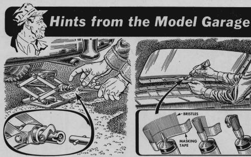
Hook Locks Jack Handle. On the usual scissors jack, the handle cross pin has an annoying habit of slipping out. A hook like this will lock the handle in place. Tighten the screw so friction keeps the hook closed while the handle turns.
