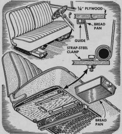
Pans Give Storage Space. To provide a place for small tools, Gladden Houck Jr., Port Chester, N. Y., installed bread pans under the seat of his Henry J. Pans 234" by 5%" by 9%" fit nicely. The pan edges slide in guides made from J-shaped tileboard molding, widened a bit by driving in drill rod.
