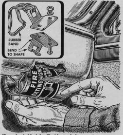
Bracket Holds Extinguisher. A can-type fire extinguisher mounted behind the dash like this can be pulled out in a hurry. The bracket is formed from two storm-sash eyes. Put them in a vise and bend as shown, making a hook on the end of one. A heavy rubber band will then keep the extinguisher in position.
