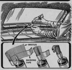
Tube Brush Spreads Cement. In applying head linings, G. E. Gannaway, Chattanooga, puts cement on with an attached brush made from paintbrush bristles. A nail inserted into the tube keeps the cement from drying out while stored.
