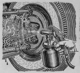
**Grease can be cleaned off** such parts as the front suspension, transmission or differential by using a paint sprayer to spray on kerosene. Allow the kerosene to soak in for a few minutes and then turn a water hose on the area full force.
