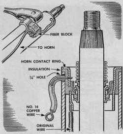
When a horn wire breaks inside the steering column, you can bypass the break by running a wire down the outside. Drill a ¼" hole in the column at the point shown. Then drill a No. 53 hole through the insulation and contact ring. Tap this for a threaded piece of No. 14 wire, insulate the wire, and connect to a junction block on the column.
