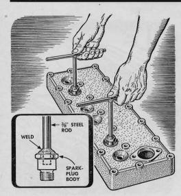
**Lifting a cylinder head** will be a lot easier if you make a couple of T-shaped handles like this. Knock the porcelain tops out of a pair of old spark plugs and weld them to handles made from %" rod. To use, screw into the plug seats.
