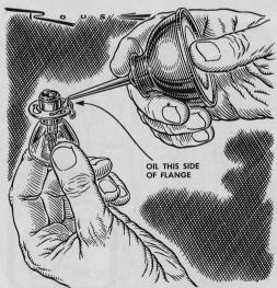
**Apply light oil** to the flange when you install a prefocused headlight bulb in an older car. This will make the bulb easier to remove when necessary. If corrosion should form, the bulb will not freeze fast to the socket assembly.
