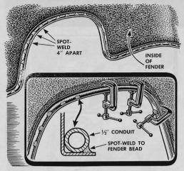
If the fenders of an old car have cracked at the edges, they can be given new strength by welding a piece of ½" electrical conduit inside the bead. The conduit will bend easily to the contour of the fender. Clamp it in place until the welding is finished. Keep the welds inside the bead to avoid damaging the finish of the car.
