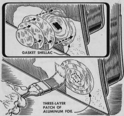
To patch a small hole in a car body, sand the metal smooth, apply gasket shellac, let it get tacky, and press down a piece of aluminum foil. Let cement harden, and cement on two successively smaller pieces. Sand edges of foil, paint patch to match.
