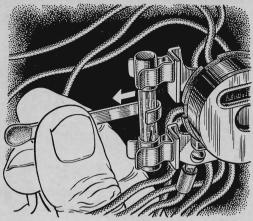
Hook Removes Fuse. Because it usually is difficult to get your fingers on a fuse, Howard Van DeWater, Kew Gardens, N. Y., suggests that garage workers make up a fuse hook. The one shown was bent to shape from a discarded wiper arm.
