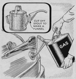
Funnel Reaches Fuel Tank. Shops that get calls to rescue gas-stranded motorists will find this funnel a useful accessory to carry along. The bent spout makes it much easier to pour gasoline into tanks with side inlets. On the cars where the filler cap is deeply recessed in a fender compartment, it eliminates wasteful, sloppy pouring.
