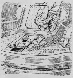
**Oil Frees Hood Latch.** After a few years, a hood latch operated by a cable running to the instrument panel sometimes sticks. You can free it by applying a light machine oil or an oil-and-kerosene mixture to the full length of the cable. The oil will penetrate the sheath. Such care may also help prevent breaks, which are hard to fix.
