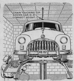
Chain Guides Lift Height. One mechanic reports that his hydraulic-lift controls are located where it's hard to judge correct car height. He fastened a chain to the ceiling. When chain touches, he stops the lift. With tall cars, he lets the chain fall over a bit.
