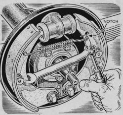
Replacing a Brake Spring. If you have trouble replacing the return spring on hydraulic brakes, try this: File a notch near the tip of an old screwdriver. Choose a combination box and open-end wrench that spans the shoes. Hook the open end over one shoe, put screwdriver through box and pry spring in place.
