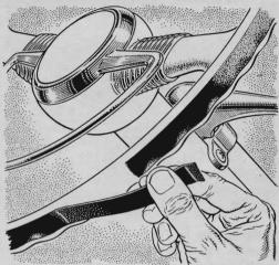
Tape Stops Wheel-Cover Slide. A steering-wheel cover that slips can be anchored by sticking friction tape around the edge of the wheel and replacing the cover. The tape's outer surface is tacky enough to keep the cover from sliding.
