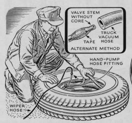
Vacuum Frees Heavy Truck Tube. To suck the tube loose from a heavy truck tire, mechanics at McElroy's Garage in Enon Valley, Pa., wrap tape around the uncored valve stem, press on the hose from the truck's vacuum brakes and run the engine. You could also hook up the wiper hose with a hand-pump hose fitting.
