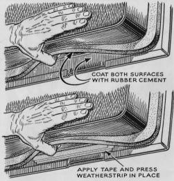
Replacing Weather Strip. When rust on the edges of a car door loosens the weather strip, try this. Coat both the strip and metal with rubber cement after brushing off the rust. Between the strip and metal, sandwich several layers of double-faced cloth adhesive tape (such as Bauer & Black Polyken No. 105). The strip will then hold.
