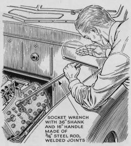
**Special Wrench for Head Nuts.** A long T-wrench made as shown here can save lots of time in removing head nuts or cap screws on V-8 engines. Use one hand as a bearing for the shank and spin the handle rapidly with the other hand.
