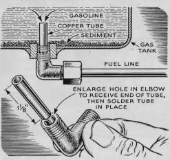
Keeping Gasoline Clean. Trucks, tractors and older cars sometimes have the outlet at the bottom of the tank. A piece of copper tubing installed as shown above will help keep dirt from the line.
