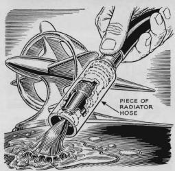
Hose on Nozzle Avoids Scratches. If you use a garden hose with nozzle to wash a car, the nozzle may slip from your hand and mar the paint. As a safeguard, slip a piece of radiator hose snugly over the nozzle. Turn this to adjust the spray.
