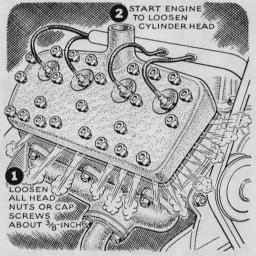
Blowing a Head Loose. Because V-type engines will run on one bank, there's a simple method to loosen stuck heads. Back off the bolts on one head about %", leave the spark wires connected, start motor, and head will blow loose. Then tighten this side down, back off the bolts on the other side and run the motor again.
