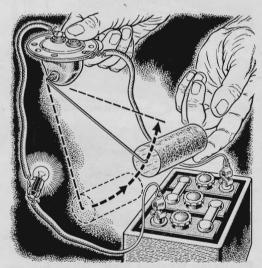
Testing Fuel-Gauge Tank Unit. You can check the rheostat in the tank unit of a fuel gauge by connecting it in series with a small six-volt bulb and then working the float arm. With the float in empty position, the light should barely glow. As you raise it, the light should steadily increase in brilliance.
