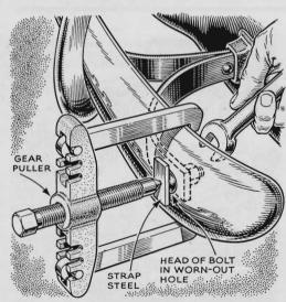
**Tightening Bumper Bolts.** If a square locking hole in a bumper has become so worn it won't hold the bolthead, assemble a two-jaw gear puller and a steel pad as shown here. (The pad keeps the puller shaft from chewing into the bolthead.) Turn the puller screw down tight and you'll be able to loosen or tighten the bolt as desired.
