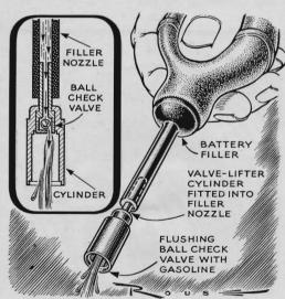
Syringe Cleans Hydraulic Lifters. If you aren't satisfied with the usual method of soaking in gasoline to clean hydraulic valve lifters, try this: Draw clean solvent into a synthetic-rubber battery syringe, fit it to the lifter stem, and force fluid through. Shake the unit as a test; the ball should make a sharp click.
