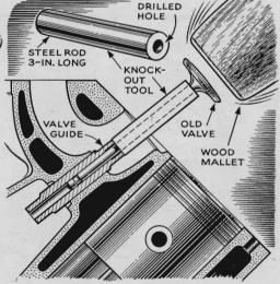
**Tool Knocks Out Valve Guides.** Worm valve guides can be removed and new ones installed in some engines by using an old valve and a piece of cold-rolled steel. The outside dimension of the knock-out tool should be slightly less than that of the valve guide, the inside drilled to the same dimension as the valve stem. Use as shown.
