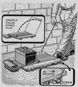
**Creeper Hauls Batteries.** Instead of toting heavy storage batteries, one mechanic moves them on a creeper fitted with a handle of ¼" cold-rolled rod. Swung down, the handle doesn't interfere with normal use of the creeper.
