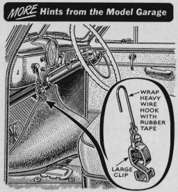
Mat Clip Leaves Your Hands Free. A clip like this will keep the mat out of the way when you're working on a master brake cylinder or battery under the floor. Hook it over one of the dashboard control knobs. A spring-closed battery clip does fine.
