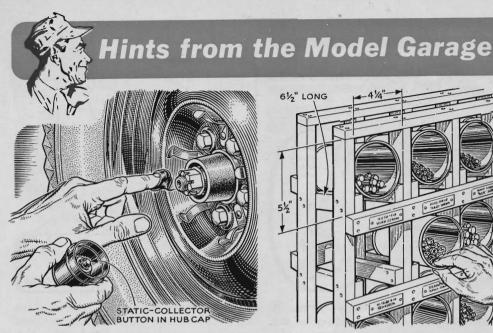
Lubricating Static Springs. When wheel springs are used to prevent static interference with radio operation, apply heavy graphite grease occasionally to the axle end. To make conductive grease, mix powdered graphite with petroleum jelly.
