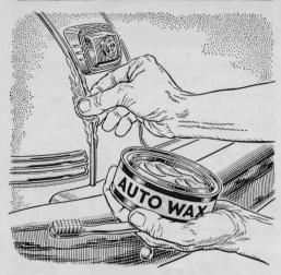
Wax in Joints Curbs Rust. While waxing your car, press a liberal amount in and around the fender welts and other joints. An old toothbrush will help force it in. Do not wipe away the wax. The excess will not be noticeable, and it serves as a good moisture seal, reducing the chances of rust forming in the joints.
