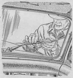
It Pays to Clean Wiper Blades. The initial smear that wipers often make when first turned on can be avoided by occasionally rubbing a soft cloth along the blades. This will remove the accumulation of grease, dirt, and oxidized rubber.
