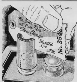
**Tag Holder for Battery Shop.** Short pieces of garden hose slotted at one end make good holders for customer identification cards in a battery-charging room. Hose of the ordinary size slips snugly over most battery posts.
