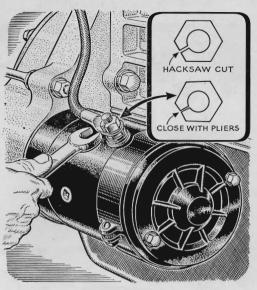
**Slotted Nut Locks on Stud.** If the threads of a stud are stripped or damaged, you can repair it temporarily by slotting a nut and squeezing it in place on the stud with a pair of heavy pliers. The same trick can be used for removing a stud with no unthreaded portion exposed. The threads won't be damaged by clamping the nut.
