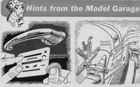
Touching Up a Scratch. A draftman's metal erasing shield is helpful for this job. Use it to limit your steel-wool rubbing to the edges of the scratch before applying touch-up paint. Use it again if you work over the area with rubbing compound.
