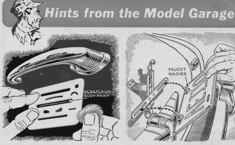
Touching Up a Scratch. A draftman's metal erasing shield is helpful for this job. Use it to limit your steel-wool rubbing to the edges of the scratch before applying touch-up paint. Use it again if you work over the area with rubbing compound.
