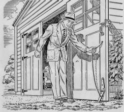
Hinge Serves as Door Stop. An old strap hinge can be used like this to keep a garage door from blowing shut. Mount it vertically with part of one leaf projecting below the bottom edge of the door. Attach a light chain to the free leaf and the door and you'll be able to lift the hinge when closing the door.
