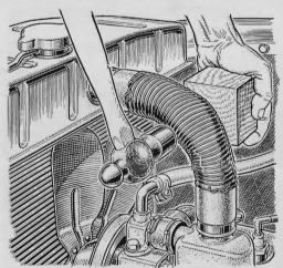
How to Curve Hose. A straight piece of rubber-and-fabric hose can be curved by wrapping it with No. 14 or 16 wire. Space the turns about \" apart and anchor the ends securely. When the hose is first curved, it may still tend to collapse, but you can make it take its proper shape by pounding with a hammer and wood block.
