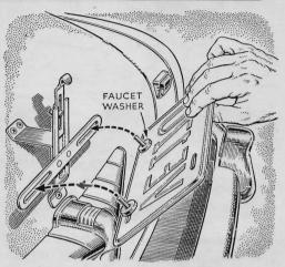
Washers Stop Rattles. A tendency of your license plates to rattle can often be overcome by mounting them with rubber faucet washers placed between the plate and bracket. Enlarge the center holes if necessary for the bolts.
