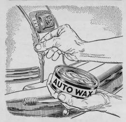
Wax in Joints Curbs Rust. While waxing your car, press a liberal amount in and around the fender welts and other joints. An old toothbrush will help force it in. Do not wipe away the wax. The excess will not be noticeable, and it serves as a good moisture seal, reducing the chances of rust forming in the joints.
