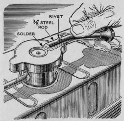
**Handle Loosens Hot Cap.** A 3" or 4" piece of iron rod riveted, soldered, or brazed to the top of a radiator cap will make it easier and safer to remove the cap when the radiator is hot. Locate the rod so it won't strike any other part of the car.
