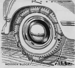
Blocks Help Put on Chains. A couple of wood blocks carried in the car will make it easier to put on your chains. Lay the chains flat on the ground, place a block between one of the cross sections, and back the car until the wheels rest on the blocks. You can then pull the chains up around the tires and fasten them more easily. The blocks must be short enough so they won't hold the chain side strands.
