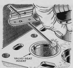
Weld Bead Loosens Inserts. Valve-seat inserts in truck and industrial engines are so hard and tough that attempts to remove them by drilling or breaking may damage the cylinder block. Such inserts can usually be removed with ease by running a weld bead around the valve-seating surface. Contraction of the weld metal shrinks the insert. Clean off any weld spatter from the top of the block or manifold passages.
