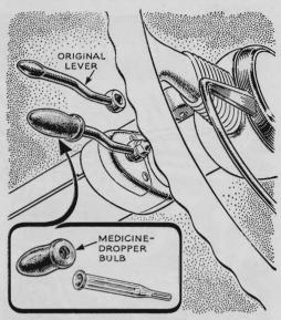
**Bulb Forms Lever Grip.** Some turn signals have a switch lever of such small diameter that your finger tends to slip off. William A. Brueske, of Wayzata, Minn., overcame this by shoving a medicine-dropper bulb over the end of the lever.
