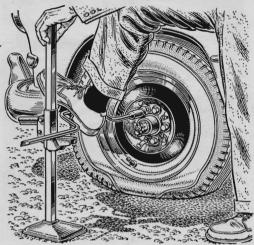
Weight Loosens Rusted Bolts. If a wheel nut or bolt refuses to budge, adjust your jack to the same height as the nut, set the lug wrench on the nut horizontally, prop it on the jack, and apply your weight to the handle. Pressure, not kicking, does it.
