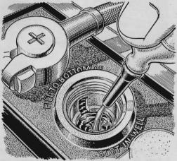
Slot Guides Battery-Water Level. In the past you were usually supposed to keep battery electrolyte just above the plates. But instructions are more specific for the latest batteries in GM cars. In these, you should add water to raise the level to a ledge at the bottom of a slot in the filler well. Don't fill above this.
