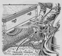
Guard Supports Trailer Hitch. A small trailer frequently doesn't have a support to keep the hitch socket free from mud and dirt when the trailer is parked. A piece of band iron bent in a half circle and welded or bolted to the tongue will give the protection needed. The loop should extend about 6" below the tongue.
