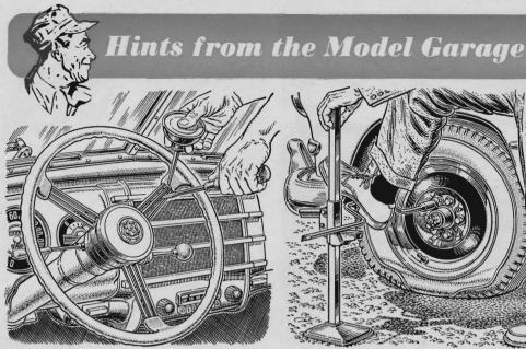
Oil Quiets Wheel Squeaks. A few drops of brake fluid or rubber lubricant will stop squeaks in a banjo-type steering wheel. Insert a screwdriver as shown and pry gently to allow the lubricant to enter where the spokes join the rim.
