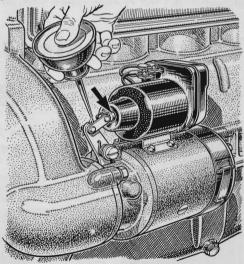
**Never Oil Solenoid Plunger.** The plunger (arrow) of a solenoid mounted on a cranking motor may look as if it needs oil occasionally—but don't apply it. Oil there will promote gum formation and coldweather sticking. Apply a little engine oil, however, to the solenoid linkage joints, as above, every 1,000 miles or so.
