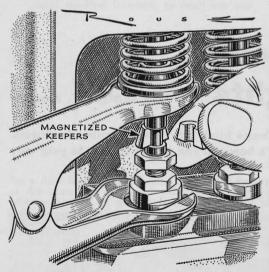
Magnetized Keepers Stay Put. A Detroit mechanic has figured out an easy way to beat the usual grease-packing method of installing valve-keepers on an L-head engine. When he takes the engine down he puts the keepers in a box with a strong magnet. When it's time for reassembly, they have enough magnetism to cling to the stem.
