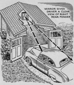
Mirror Guides You In. If you must angle into a narrow garage, install an old mirror on the back wall of the garage so that you can watch the right side of the car. A dark board mounted outside a window pane will often substitute for the mirror.
