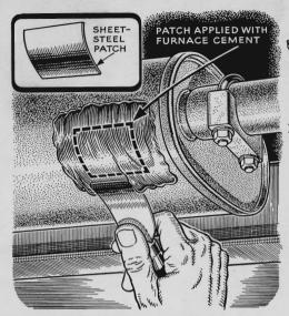
One Way to Repair a Muffler. You may save the price of a new muffler by using a little furnace cement. Clean the area and cement a steel patch over the hole. Don't start the engine until it dries. The repair may extend muffler life a year or more.
