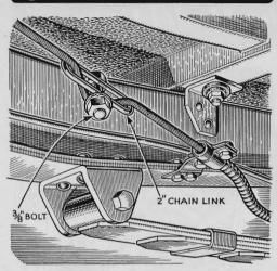
**Tightening a Brake Cable.** In some cases, you can take up slack in a parking-brake cable as shown here. Be careful to locate the chain link and bolt in a free area so that they will not interfere with the travel of the brake cable.
