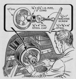
Homemade Wheel Puller. Find an old wheel that will fit the car and burn off the rim with a torch, leaving just the center disk. Weld the pipe to it, the cap to the pipe, the nut to the cap, and the handle to the screw head. To pull a drum, remove the wheel nut, attach the disk, and turn the screw against the spindle.
