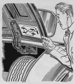
Rotation Chart Guides Mechanic. Different garages may rotate tires in different patterns. To make sure yours are transposed in the same way each time, cement a diagram under the trunk lid. Instruct the mechanic to follow this pattern.
