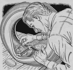
End Wrench Spreads Tire. It's difficult to apply a patch to the inside of a tire casing without a tire spreader. As a handy substitute, take a large open-end wrench and prop the sides of the casing apart as shown in the drawing above.
