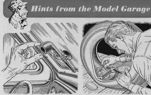
A Pipe Rack in Your Car. A piece of inner-tube rubber between two suction cups on windshield or dash makes a convenient pipe rack. Use cups with threaded shafts. Make holes in the rubber, slip it on the shafts, and tighten the nuts.
