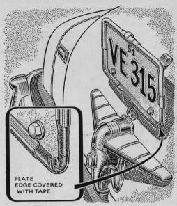
**Tape Tightens License.** If a license plate rattles in an ornamental frame, you can make it fit snugly by placing friction tape around the edge of the plate. The tape won't be noticeable if you fold the excess over the back.
