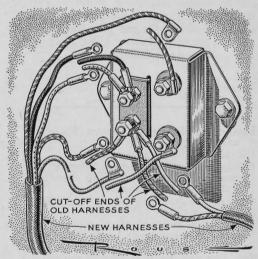
**Out With Those Old Wires.** You can install a new wire system in a car easier and faster if you first cut the old wires a couple of inches from the terminals. Then remove the old harness and install the new. Finally, use the color code on the old wire stubs as a guide in attaching the new ones. Remove one stub, then attach new wire.
