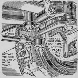
Twisting Makes Grease Go In. If grease does not come out at the indicated point when you are lubricating tie-rod ends, put a pipe wrench on the rod and twist it gently, first one way and then the other, until grease appears. Never force the grease too much, or you'll drive out or buckle the bottom plate, ruining the end.
