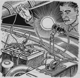
Trouble Lamp Easily Made. Most autosupply stores carry frosted six-volt bulbs in 15- and 25-watt sizes with a base like ordinary house bulbs. With one of these, you can quickly make an efficient trouble lamp for your car. A standard socket, some sort of clamp, wire, and alligator clips are all you need.
