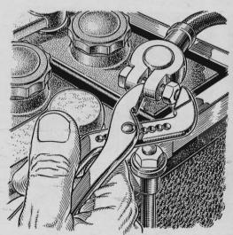
Pump Pliers Loosen Cable. If you own a pair of water-pump pliers, they can do double duty in removing battery cables. Loosen the cable clamp nut about two turns, put on the pliers as shown above, and squeeze and twist at the same time. The jaw of the cable clamp will loosen on the terminal as you squeeze the pliers.
