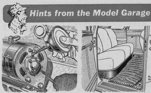
Brush Cleans Oil Holes. To clean out oil holes and keep grit out of bearings, solder a bent mucilage brush to the spout of your oilcan. A few swipes of the stiff brush will sweep away accumulated grime before you squirt oil into the holes.
