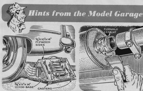
Tool Dolly a Big Help. A mechanic lying on a creeper can keep his tools handy with a low dolly like this. Use the triangular space inside for rags, pump oilers, and the like. The dimensions shown make a dolly of a convenient size.
