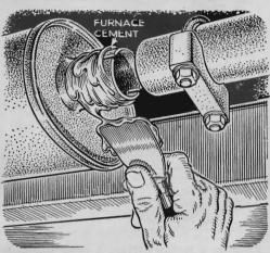
Cement Seals Tailpipe Joint. In fitting a tailpipe to a muffler, you can get a better seal by applying a little furnace cement before slipping the units together. A 20-cent can of cement is enough for a dozen or more such jobs.
