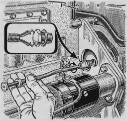
Grabbing Tool Saves Plug. If you've ever filled a Hudson wet clutch, you know how easy it is to drop the plug inside the housing -and how difficult it is to get out. Some mechanics stuff in a rag to catch it, but here's a better way: Buy a flexible grabbing tool like the one shown and use it for this job.
