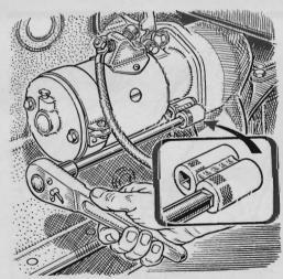
Offset Socket Turns Nut. In loosening or tightening starter bolts on some cars, you can't use a socket wrench because there's no room for the handle. For such jobs, Marion L. Rhodes, Knightstown, Ind., welded two sockets together side by side. With these and an extension rod, he can take a half turn at a time.
