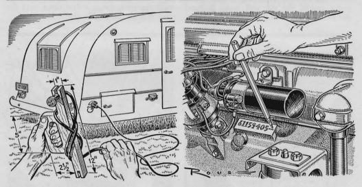
Reel Stores Extension Cord. House trailers are often equipped with 115-volt electric wiring circuits, but to bring current into the trailer a long and unwieldy extension cord is required. To simplify handling the cord, A. V. Malone, of Los Angeles, designed this carrier. Wind the cord as shown, each revolution forming a figure eight. The 1" slots at each end are for hooking the plugs to the carrier.
