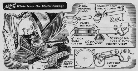
Glass Magnifies Map Details. A large reading glass mounted under the dash like this will help you see fine print on a highway map. Supported on a pivot, the glass swings into a pocket lined with foam rubber while not in use. This protects the lens
