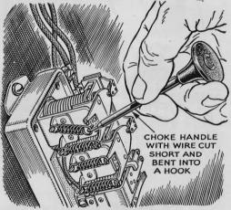
**Choke Handle Is Spring Tool.** Here's an easily made tool that Marion L. Rhodes finds handy around his shop in Knightstown, Ind. It's just the thing to hook on or off the small springs in a current and voltage regulator. Carburetor and generator springs are other possible uses. The wire is stiff enough to retain its hook shape.
