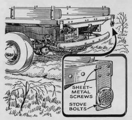
**Swinging Reflectors Escape Damage.** If you should back your truck into an obstacle, flexibly mounted reflectors will swing under the truck bed without damage. Bolt each reflector to a piece of canvas belting about 12" long and attach the other end of the canvas to the truck bed with nails or self-tapping metal screws.
