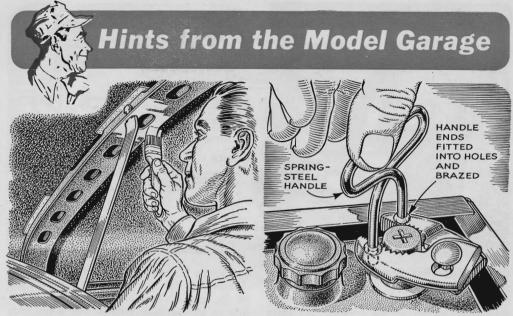
White Paint Shows Brace Slot. In the dark it's often difficult to prop up your hood with a swinging brace because you can't see the slot. Applying a little white paint around the slot will make it stand out prominently even in poor light.
