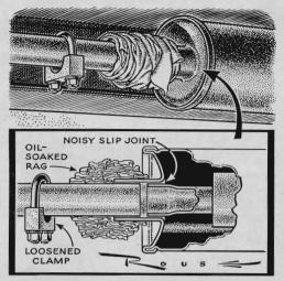
**Oil Quiets Noisy Muffler.** If noises come from a muffler slip joint, wrap the joint with cloth, saturate with penetrating oil, and leave overnight. If this fails, remove muffler and apply the oil. The oil cleans out rust that keeps joint from slipping properly when temperature changes expand or contract the inner muffler tube.
