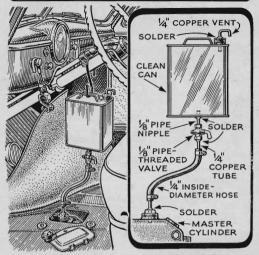
Bleeding Hydraulic Brakes. This rig will make it easy to bleed your brake system after a repair job. To assemble it, you'll need a spare cap for the master cylinder. Solder a piece of ¼" tubing into a hole drilled through this cap. You can also use the assembly to flush the brake system with alcohol.
