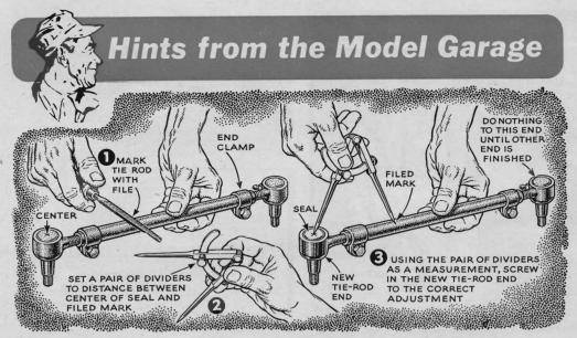
**Replacing Tie-Rod Ends.** When worn tierod ends are replaced, the following procedure will make it unnecessary to realign the wheels after the job is done.
